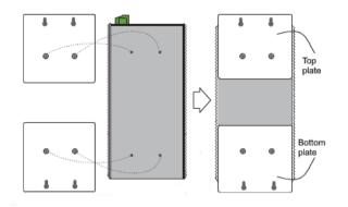
Step2: To install the switch on the wall, 4 screws are required for wall mounting.
