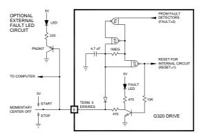
At anytime the operator can push the switch to the "STOP" position to immediately halt the G340 drive. Anytime the G340 is in the "FAULT" state (FAULT LED lit), all switching action stops and the motor freewheels and is unpowered. This will light the "FAULT" light.
