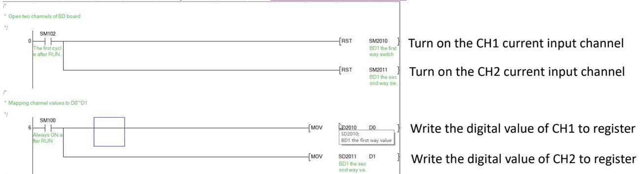
2. Programming example using "BD module configuration" function of host computer software:
